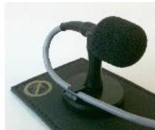
**Recommendations :** pinch the cable through the cable guide. It minimizes the movement of the cable around the microphone.
