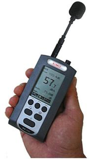
**Important :** the D-MB microphone must be connected on channel 1 for a hand sound level meter use
